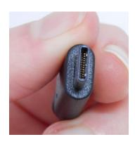
On the right side of Vario 440 you can find the USB port, which is USB type C. Special about the USB Type C port is, that it doesn't matter which direction the USB plug is facing. No more finding the right position of the plug.
