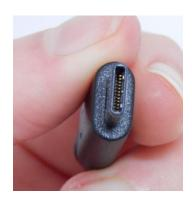
On the right side of Vario 480 you can find the USB port, which is USB type C. Special about the USB Type C port is, that it doesn't matter which direction the USB plug is facing. No more finding the right position of the plug.
