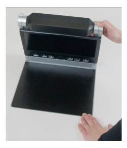
Lift arm until you feel it snap into position. **Warning:** To avoid touching the camera window, do not lift from the camera housing!
